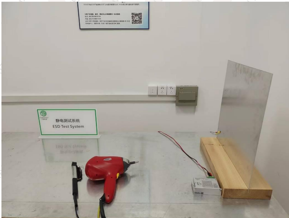
Photographs 2: Set-up for Electrostatic discharge (ESD)
